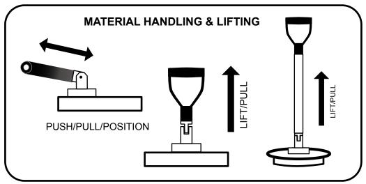
MULTI-GRAB III series tools have all the design features and functionality of the MULTI-GRAB II series tools with the exception of a stainless steel locking pin. Pull ring to disengage pin. Twist ring to rest in detent for free pivot of handle. Twist ring and align with slot to allow pin to lock into a hole in either straight position or 90 degrees. **LOCKING PIN**
