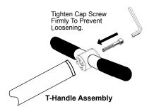
The T-Handle comes packaged with a hex head cap screw already inserted into the handle bar. Fit the handlebar so that it seats into the grooves on the end of the main tube. With the included 1/4" hex key, tighten the hex head cap screw firmly so handlebar is locked into position. A firmly tightened bolt will prevent loosening during use. Check periodically to make sure hex head cap screw is tight.
