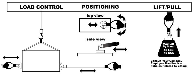
Note: Examples are shown with a MG003 & MG004-36 as the tool being used. All of the MULTI-GRAB products function similarly but have different features. See the back of this sheet for more information and details on the features of each model.
