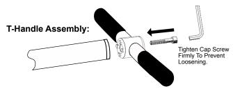
The T-Handle comes packaged with a hex head cap screw already inserted into the handle bar. Fit the handlebar so that it seats into the grooves on the end of the main tube. With the included 1/4" hex key, tighten the hex head cap screw firmly so handlebar is locked into position. A firmly tightened bolt will prevent loosening during use. Check periodically to make sure hex head cap screw is tight.
